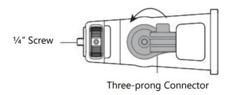
**Tip:** You can adjust the angle of the three-prong connector on the base by loosening or tightening the screws to get the desired camera angle.
