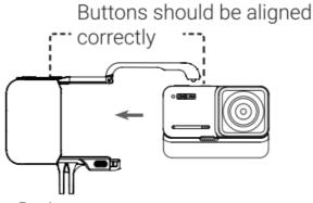
5. Insert ONE RS into the Mounting Bracket
