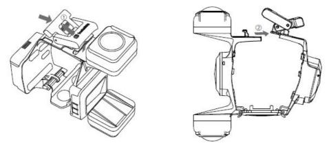
2. As shown below, lock the mounting bracket's connection buckle onto the bottom of the drone.
