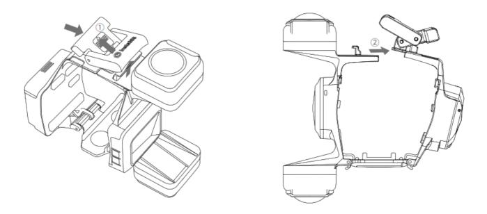
**Step 2:** As shown below, lock the mounting bracket's connection buckle onto the bottom of the drone.
