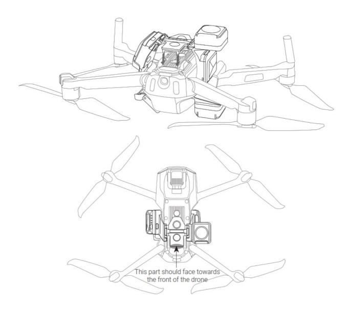
Step 3: Lock the Lock Lever well and ensure that the yellow mark of the Lock Lever is not showing.
