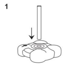
13. Attach the connecting frame to the rod.
