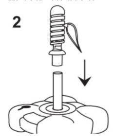
10. Attach a carabiner with a ball to the eyelet.
