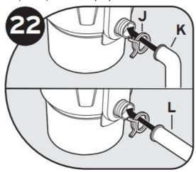
Place tube (K or L) into Anti-Vibration Tailpipe Mount<sup>TM</sup>. Use provided tubes for best results. Secure with spring load hose clamp (J) (provided).
