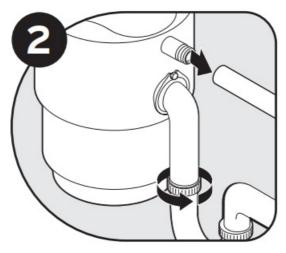
Turn off electrical power at circuit breaker or fuse box. Disconnect drain trap from waste discharge tube. Disconnect dishwasher if connected to the disposer.
