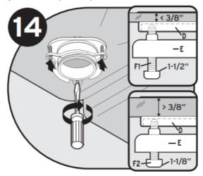
Tighten 1-1/2" screws (F1) evenly and firmly against backup flange. Use shorter 1-1/8" screws (F2) if sink is more than 3/8" thick.
