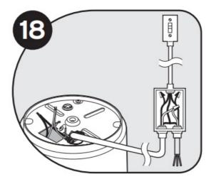
This disposer requires a switch with a marked "Off" position (wired to disconnect all ungrounded supply conductors) installed within sight of the disposer sink opening (1 hp minimum rating).
