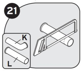
You may need to trim discharge tube (K or L) to ensure proper fit.
