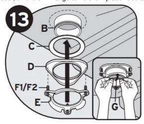
Insert fiber gasket (C), backup flange (D) and mounting ring (E). Hold in place while inserting snap ring (G). Pull snap ring (G) open and press firmly until it snaps into place.
