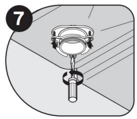
Using a flathead screwdriver, loosen the 3 screws on the mounting assembly.
