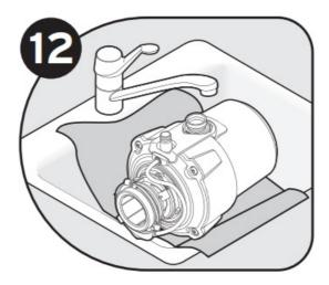
Place a weight, such as the disposer, on the sink flange to hold it in place. Use a towel to avoid scratching sink.
