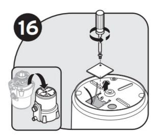
Turn disposer over and remove electrical cover plate. Pull out wires.
