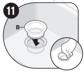
Press flange (B) firmly into sink drain. Remove excess putty.
