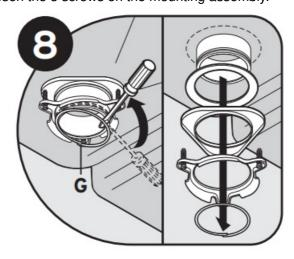
Using a flathead screwdriver, pry off the snap ring (G).
