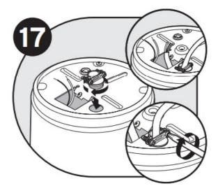
Insert cable connector (not included) and run electrical cable through access hole on bottom of disposer. Tighten cable connector.
