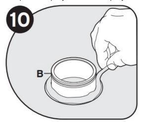
Evenly apply 1/2" thick rope of plumber's putty around sink flange (B).
