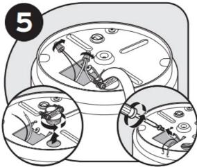
Disconnect the disposer wires from the electrical supply. Is the new disposer mounting the same as the old one? If YES, you may choose to skip to step 15.
