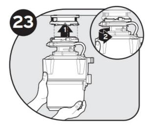
Lifting disposer from the bottom (1), hang disposer by aligning 3 mounting tabs with slide-up ramps on mounting ring and (2) slightly turn disposer clockwise.
