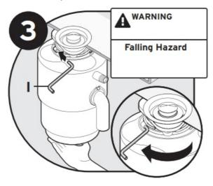
Support disposer, insert end of wrenchette (I) into right side of mounting lug, and turn. Disposer will fall free.
