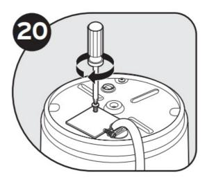
Push wires into disposer and replace electrical cover plate.
