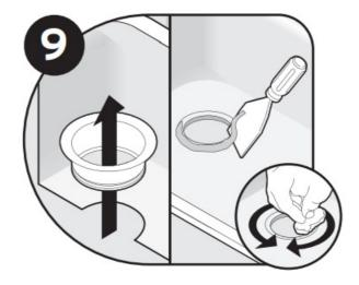
Remove flange from sink. Remove old plumber's putty from sink with putty knife.
