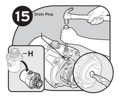
Turn disposer (H) onto side and knock out drain plug with screwdriver. Remove plug from inside of disposer with pliers.
