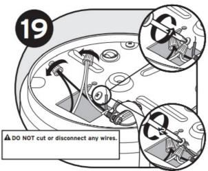
Connect white wire from disposer to neutral (white) wire from power source. Connect black wire from disposer to hot (black, red) wire from power source with wire nuts (not included). Connect ground wire to green grounding screw. Unit must be grounded for safe and proper installation.
