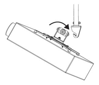
4. Tighten the screws on both sides of the mount base to hold it in place
