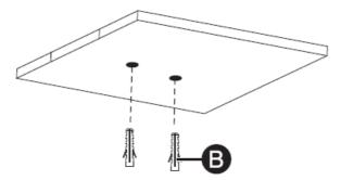
4. Attach the ceiling plate (K) to the concrete ceiling using the wood screws (A) provided, then tighten the screws **CAUTION**: DO NOT over-tighten the screws.
