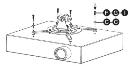
3. Tighten the four screws used to attach the arms to the mount base in step 1.
