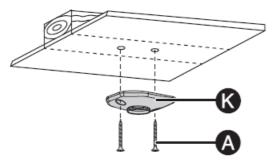
STEP 1 – Option 2: Mounting to a concrete ceiling
