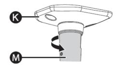
2. Tighten the set screw at the top of the mount body using the Allen key (J) from the hardware kit.
