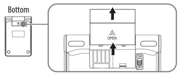
2. Insert the included AAA battery into the battery compartment. Make sure that the + and – signs match the symbols in the compartment.
