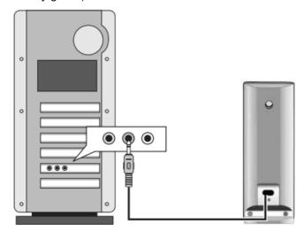
3. Plug the cable with the black plug on the right speaker into the jack on the subwoofer.
