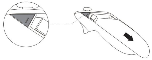
2. Install the rechargeable battery pack making sure you have it aligned with the correct polarity. Slide the custom battery door onto the controller.
