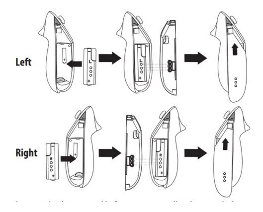
\* Grips need to be removed before using controller charging dock.
