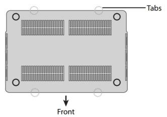
4. Open your MacBook about halfway and make sure that the tabs on the top cover are placed near the bottom of the screen.
