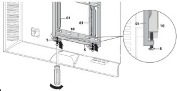
Tighten the locking screws (S) with a Phillips screwdriver until they contact the wall plate (10).
