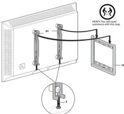
**Securing the TV to the wall plate**
