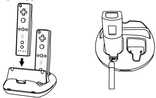
2. When inserting the Wii Remote into the charge station, the charge status indicator glows red while the battery pack is recharging. When recharging is complete, the charge status indicator glows green.
