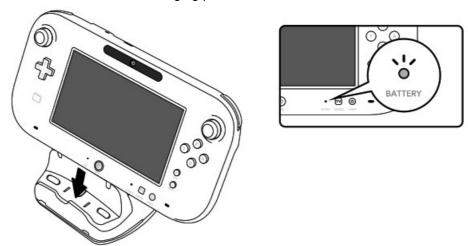
2. The Battery LED on the Wii U GamePad lights up orange during charging and will turn off when the battery is fully charged.
