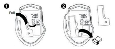
3. Insert the included AA battery into the battery compartment. Make sure that the + and – signs match the symbols in the compartment.
