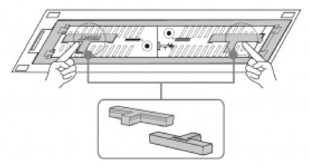
3. Attach the rubber locks to the stand using the lock that matches the marking shown in the illustration below. Note
