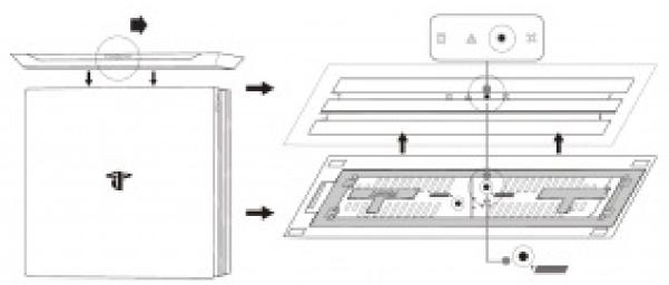
7. Use the mounting screw to secure the vertical stand to the bottom of your PS4 Slim game console. Tighten the screw with a coin or flat blade screwdriver.
