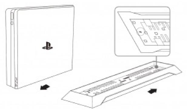
3. Remove the mounting screw and the adapter from the bottom of the vertical stand.
