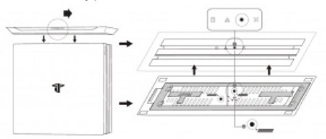
Use the mounting screw to secure the vertical stand to the bottom of your PS4 Pro game console. Tighten the screw with a coin or flat blade screwdriver.
