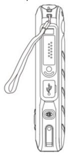
6. Installing headset Open the cover from the top of the device to show the headset sockets. The headset will work immediately after being plugged in.
