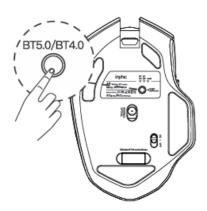
(2) Press the button to switch to the desired BT mode
