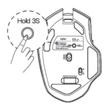
(3) Long press for 3 seconds, the indicator light flashes quickly and enters the pairing mode
