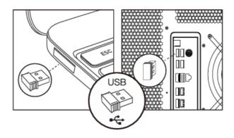
(2) Plug the receiver into the interface of the device
