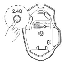
(4) Press the MODE button to switch to 2.4G mode (red light) to use
