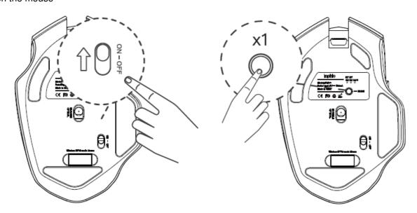
2. Press the button to switch to the desired BT mode (BT 5.0, the green light flashes slowly; BT 4.0, the blue light flashes slowly)
