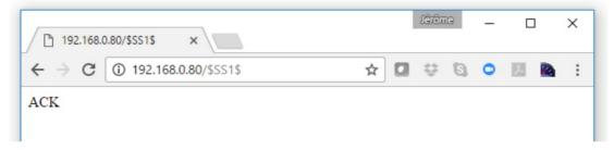
You can also use any telnet application in order to communicate with the device using TCP. Make sure to use the right IP address and **port 50000**.
