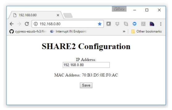
You can use the commands by sending HTTP or TCP requests. For example, you can send an HTTP request by sending it using any browser to 192.168.0.80/COMMAND. If the command is recognized, you will receive the ACK string.
