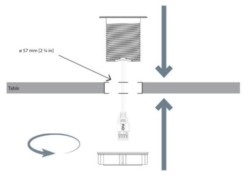
2. Use a CAT cable with the appropriate length and connect the terminal block to the CAT conductors according to the TOGGLE ROOMS GPI connection.
