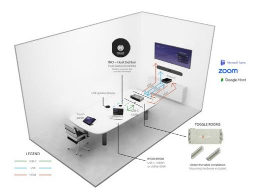
The button acts as a trigger to enable laptop/BYOM mode for TOGGLE ROOMS.
