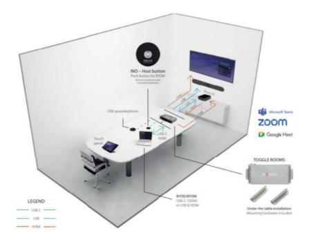
The button acts as a trigger to enable laptop/BYOM mode for TOGGLE ROOMS.
