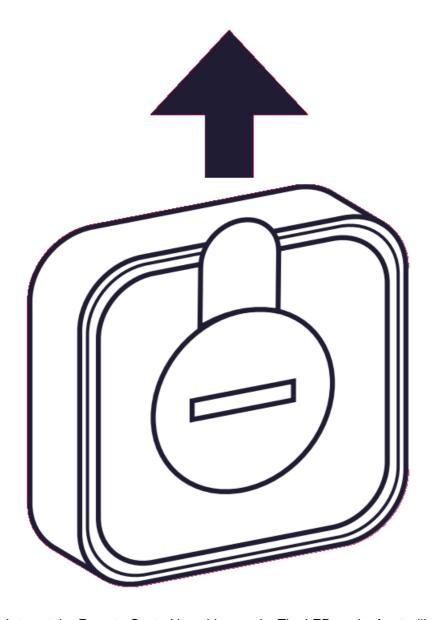
Remove the plastic tab to put the Remote Control in pairing mode. The LED on the front will start blinking once per second.\*
