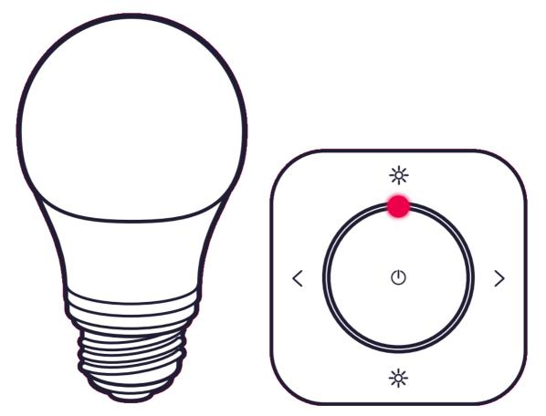
Bring the Remote Control close to the light (< 10cm). The light will blink to confirm it's successfully connected. Repeat Step 2 for all lights that you want to connect to the Remote Control
