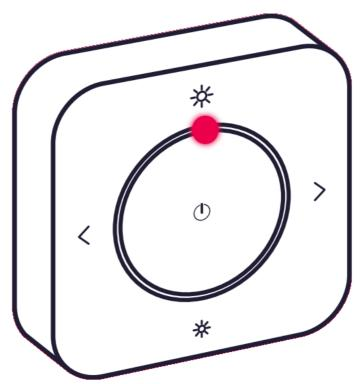
Press the button in the middle together with the top button (big sun) and hold for 3 seconds. The LED will start blinking once per second.
