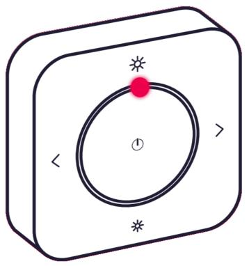
The LED will rapidly blink twice to confirm it's successfully connected. **NOTE:** the Remote Control will not appear in the Philips Hue app.
