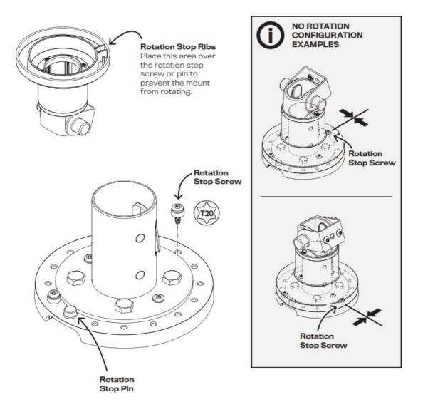
3. When placing the top of the mount onto the base, ensure the rotation stop ribs fall in between the rotation stops that were set in place in Step 2. Or in a no-rotation configuration, the ribs must be placed over top the rotation stop screw or pin.
