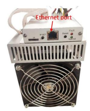
**Normal Indicator:** Being constantly lit represents static IP and flickering represents DHCP **Fault Indicator:** Being on means there is something wrong with the network; Being off means it is OK.
