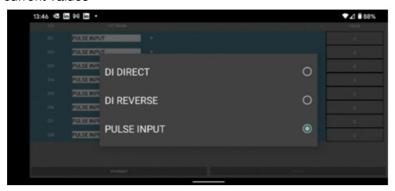
Use the drop-down arrows in the "I/O Mode" column to select the type of input type by clicking in the respective radio button –
