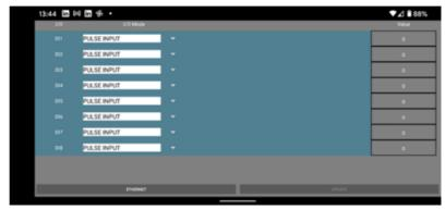
Once connected, you will land on the I/O setup screen, where you can set up the I/O and read input and output current values –
