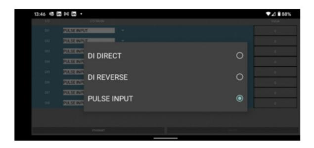
Use the drop-down arrows in the "I/O Mode" column to select the type of input type by clicking on the respective radio button –
