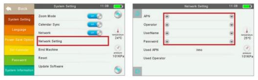
• The GPS and Network functions are switched on by default. You can change the connectivity options in "System Setting" -> "Network ON/OFF" and "GPS ON/OFF".
