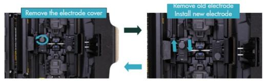
Clean the new electrodes with alcohol-soaked clean gauze or lint-free tissue, and install them in the splicer.
