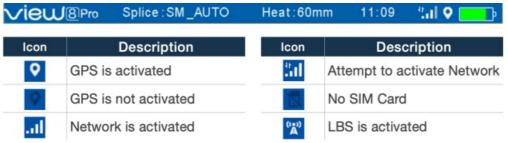
• If the network activation fails, go to "Network Settings" and enter the APN details manually. Refer to your SIM card provider for the correct APN details
