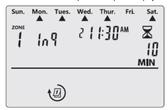
**Turn On/Off:** Turn on to enter the auto mode to irrigate based on programmed schedules; turn off to immediately cancel all progressing irrigation and, also forbidden auto irrigation.
