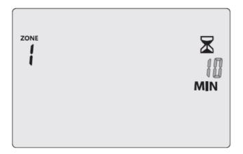
Display in Manual Irrigation Process: the screen displays the serial number of the current irrigation zone, the remaining time and the current date and time.
