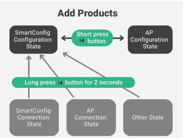
Power on the device, reset the Wi-Fi network and choose the connection mode.
