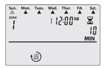
Press the + or - button to activate or forbidden irrigation on the designated day which is flashing, then move to the setting of the next day. Or you can press the button to move to the setting of the next day.
