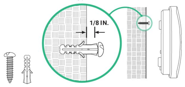
• You can tighten up both holes on the bottom using screws just in case, though it would be uneasy to disassemble them afterward.
