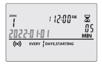
Press the button button to quit setting and reverse back to automatic mode. The device will automatically quit and go back to automatic mode, if there is no operation within 10 minutes.
