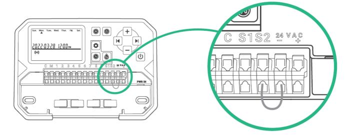
Separately connect the 2 lines of the rain sensor to ports 24 VAC- and S1 (or S2).
