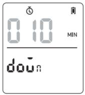
**Step4:** Press the OK button or no operation for 30 seconds to confirm and save the set parameters.
