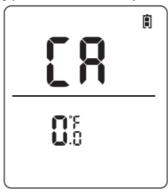
**Step2:** Press the +/- button to adjust the parameter value to 0.5°F.
