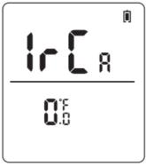
**Step4:** Press the +/- button to adjust the parameter value to 1.0°F.
