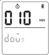
**Note:** After the countdown starts, we can press the +/ button to adjust the countdown time, then press the OK button to confirm and restart the countdown with the adjusted duration, or no operation for 10 seconds to resume the countdown before adjustment.
