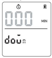
**Step2:** Confirm that the screen displays "Down". If not, press and hold the DONENESS button for 2 seconds to toggle the display.
