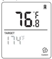
**Step3:** Press the OK button or no operation for 30 seconds to confirm and save the set parameters.
