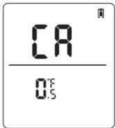
**Step3:** Press the MEAT button to display "IRCA" on the screen to set the calibration value of infrared temperature. Meanwhile, the corresponding parameter flashes.
