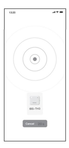
The phone app will automatically scan and find the device. Once the device is found, confirm and click "Next Step" to continue.
