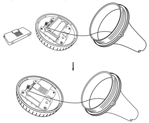
• Make sure the silicone waterproof ring is well placed, then close and tighten the lid of the pool thermometer.
