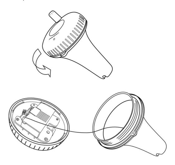
• Remove the battery cover, install 2 AAA batteries, put the cover back.
