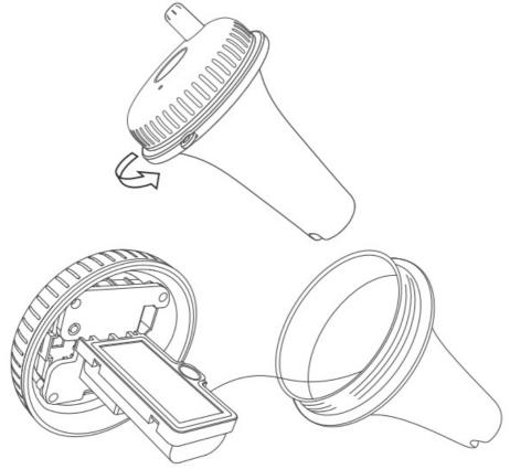
• Remove the battery cover, install 2 AAA batteries, put the cover back.
