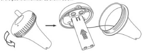
Remove the battery cover, install 2 AAA batteries, put the cover back.
