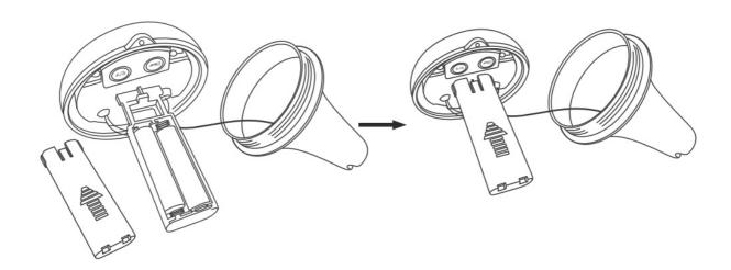
• Make sure the silicone waterproof ring is well placed, then close and tighten the lid of the thermometer.
