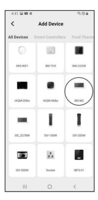
3.3.2 Plug into a USB power supply, power on properly, and click Next Step to continue.
