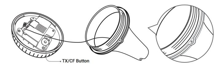
⚠ The green part is a waterproof gasket, which should not be removed at any time!
