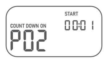
Briefly press the button to select the Countdown ON mode, which displays COUNT DOWN ON and P02 on the left and START 00:01 on the right.
