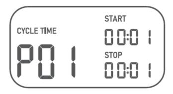
• Briefly press the button to select the Cycle Time mode, which displays CYCLE TIME and P01 on the left, START and 00:01 on the top right, and STOP and 00:01 on the bottom right.
