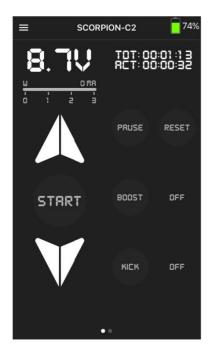
7. When a powerpack is added you can Press "Back" to access to the run page(s). To select the powerpack you want to control (when two or more powerpacks are paired) you can tilt the powerpack (recommended) and the run page will automatically change. You can also manually swipe pages to select device. To access the settings page press the 3 lines in the upper left corner.
