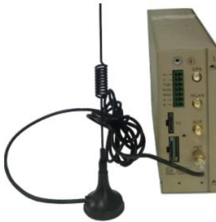
Figure 3-6 Installing an Antenna
