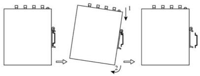
Figure 3- 2 DIN rail disassembly schematic diagram
