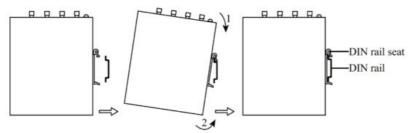
Figure 3- 1 DIN rail installation schematic diagram
