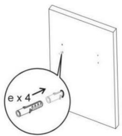
**Step 5**Turning 4pcs screws c into 4pcs e to fasten a by screwdriver. As shown below:
