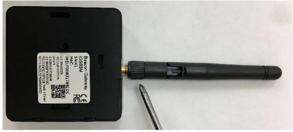
2. Step 2. Remove the screw from the bottom cover
