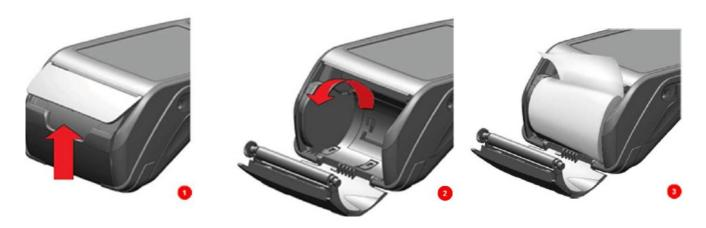
Hold the terminal securely in one hand. With the other hand, and by using two fingers, lift the printer cover release as shown. Fully open the printer cover and remove the old roll of paper.
