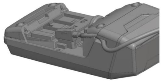
• Close the tap door and ensure the cable doesn't block the door.
