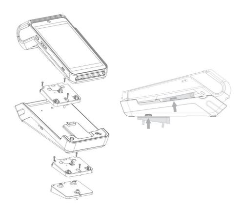
If removal of the base and DX8000 is required, use screwdriver to push the area of the structure to unfix them.
