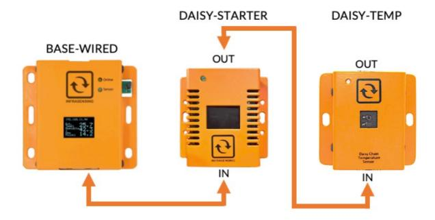
4.4. If you would be connecting another Daisy Sensor to the chain, you just have to connect the OUT port of the first Daisy Chain Sensor to the IN port of the next Daisy Chain Sensor. It should look like this sample:
