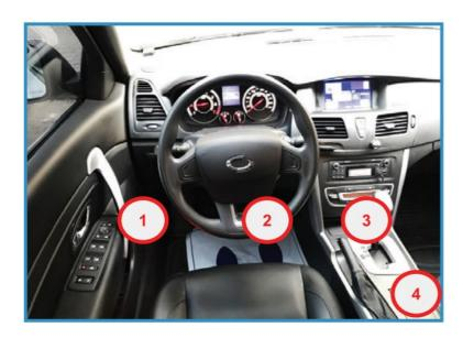
When the car is turned off, attach the terminal to OBD socket shown above, and start the car (red LED light is up when installed normally). Fuse box and terminal box should be removed from the cover. If the OBD socket is located on a pedal or other location that you cannot see, please use a flash for installation. Location of OBD socket may vary depending on vehicle's manufacturer and model.
