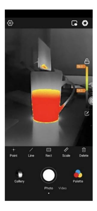
The isotherm scale can be used for palettes other than white-hot or black-hot to highlight the temperature zone requiring special attention. The selected zone is displayed in the form of a palette while others are white-hot. To clear all the points, lines, and frames, tap the rightmost **Delete** control.
