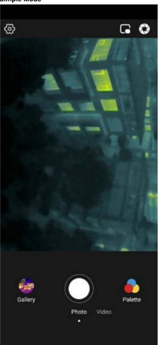
In Simple Mode, users can see the infrared image, and the functions of photo taking, video taking, galleryand palette replacement are supported.
