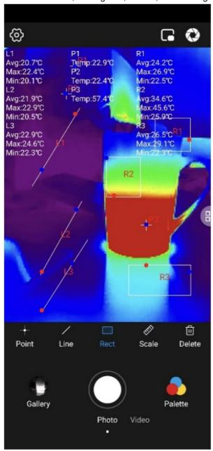
Only point-based temperature measurement supports adding or dragging measurement points. To delete a measurement point, tap the point. This is also the case for other controls.
