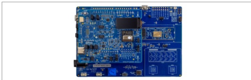
Figure 2 SHIELD_XENSIV_A XENSIV™ sensor shield connected with CY8CKIT-062S2-43012
