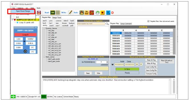
Load configuration into the current board by selecting "write to Device 0x01"
