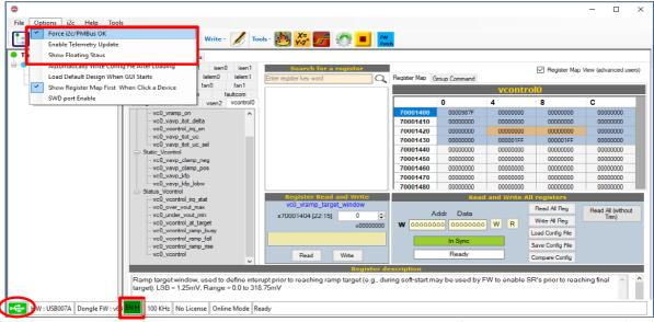
The I2C communication can also be enabled by checking "Force i2c/PMBus OK" undre option. The I2C status button on the register map page indicates "In Sync" in green. Select "Force I2C/PMBus Ok" to force the the communication on defult address from the option menu. "Enable Telemetry update" and "Show Floating Status" must to be enabled aswell. The Enable signal from I2C needs to EN H as well.
