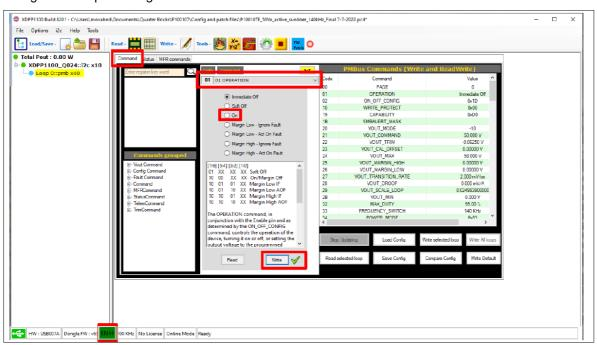
• Click on "Loop 0::pmb x40", click on "Status" tab, and Adjust "39 IOUT\_CALIBRATION\_OFFSET" under "PMBus Commands (Write and ReadWrite)" to achieve less than 0.25 A at no load on the Telemetry. Make sure to click on write after each adjustment to see the effect in telemetry.
