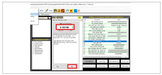
• After the IOUT is trimmed to match the load, the configuration file is ready to be burn into the IC. Open the "Multi Device Programmer". For a single configuration, use the default "Xvalent=0". Click the "Program Configuration to OTP" button to store both I2C and PMBus configurations to OTP.
