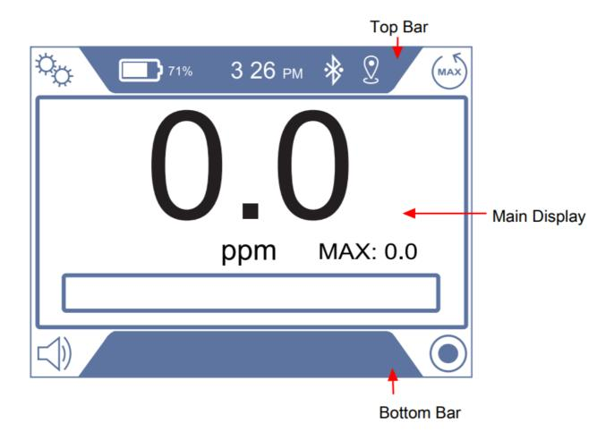
Top bar: The top bar includes the battery symbol and charge %, time, GPS, and bluetooth status.
