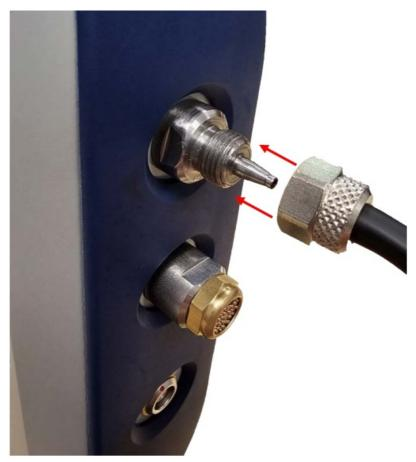
2. Hand-tighten the nut. Be careful not to over-tighten.
