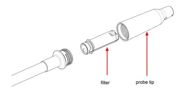
Exposing the filter to water or oil can block air flow. If this occurs, first disconnect the disc filter to release any vacuum in the sample tube. Then remove the filter with the unit turned off and the probe facing down to avoid getting contaminants in the probe and install a new filter. If the filter is wet, it can be reused once it dries.
